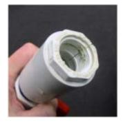
In a threaded joint the greatest stress is generated within the meshed threads; so any cracks or failures will originate from the interior and progress to the exterior. The wall thickness of the female threaded portion, part or assembly has an insignificant effect on preventing failure from cracking.
