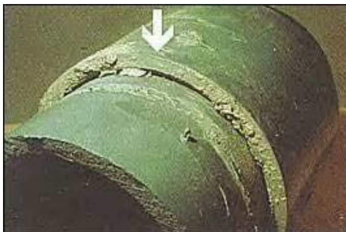
Figure 22: Insufficient Solvent cement was used.
