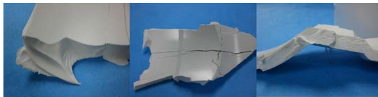
Figure 1: Typical burst or short term failure
