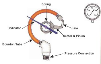
gauge shows a rare flicker, it may be ignored or overlooked. However, high activity of the pointer calls for further investigation. Systems are designed and intended to run with a steady working pressure. An unstable needle reflects the presence of destructive changes in the system pressure.
