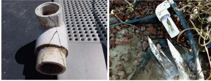
**Figure 7: Breaks due to freezing water**
