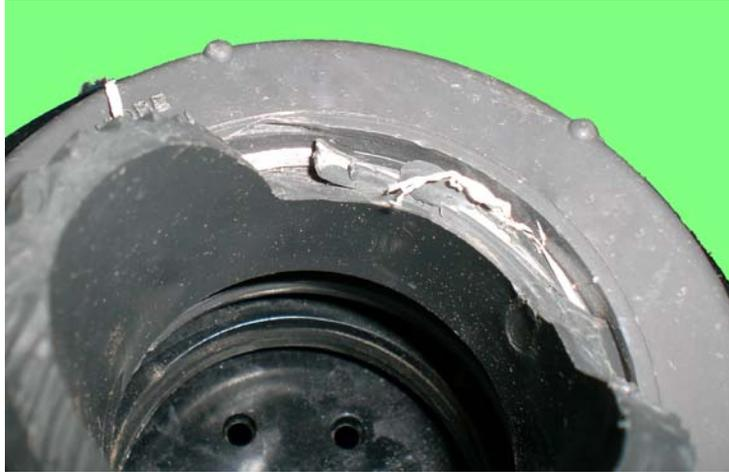
**Figure 9: Vibration failure of male threads.**
