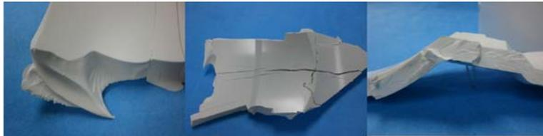
Figure 1: Typical burst or short term failure
