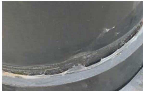
**Figure 12: Assembly was moved during cure time.**
